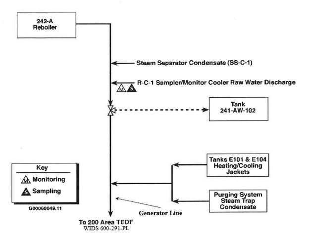
Figure D-1. 242-A Evaporator Steam Condensate Flow Schematic.
